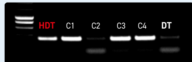
Performance test on a difficult template: Hot Diamond Taq® (HDT) & Diamond Taq® (DT) were evaluated against HotStart competitors (C1, 2 & 4 - Chemical modification ; C3 - Antibody) for their ability to amplify a difficult PCR template (gDNA NUMB - 306b). PCR products were analysed by gel electrophoresis.
