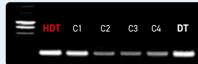
Performance test on a 72% GC rich template: Hot Diamond Taq® (HDT) & Diamond Taq® (DT) were evaluated against HotStart competitors (C1, 2 & 4 - Chemical modification ; C3 - Antibody) for their ability to amplify a GC rich PCR template (SC03449 - 152b). PCR products were analysed by gel electrophoresis.
